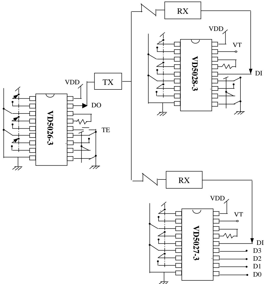
The IC substrate should be connected to  $V_{DD}$ . 芯片襯底請接  $V_{DD}$ 。
