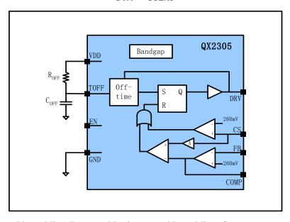
The T<sub>OFF</sub> can be reduced by adding R<sub>OFF</sub> and be increased by adding C<sub>OFF</sub>.
