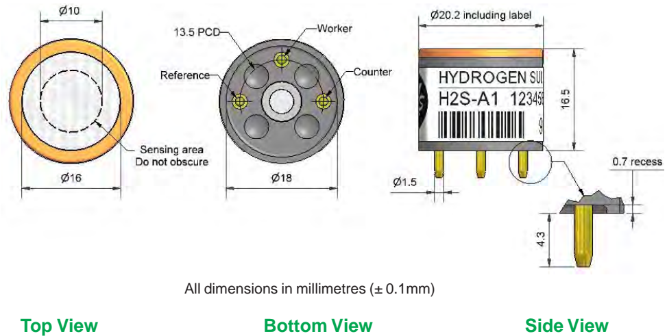
Figure 1 H2S-A1 Schematic Diagram
