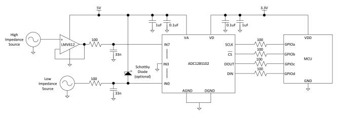
Figure 38. Typical Application Circuit
