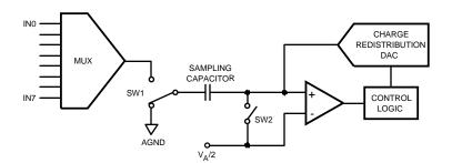
Figure 35. ADC128S052 in Hold Mode
