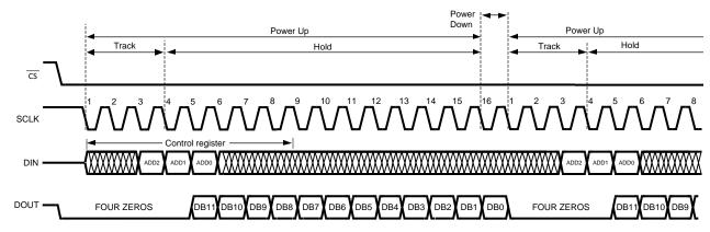
Figure 1. ADC128S052 Operational Timing Diagram
