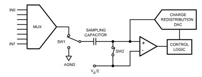
Figure 34. ADC128S052 in Track Mode
